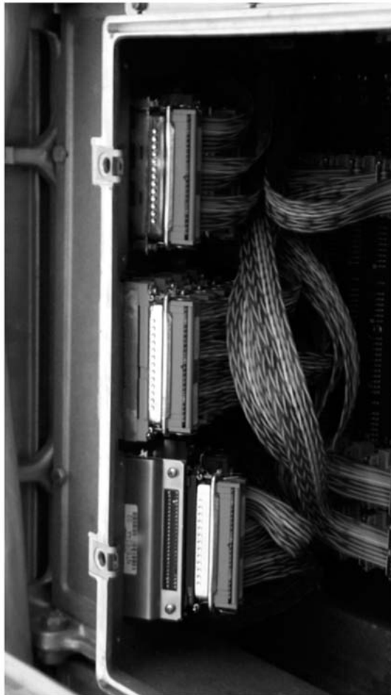
Figure 5: Install adapter 50-pin connector in backplane 50-pin cable connector
